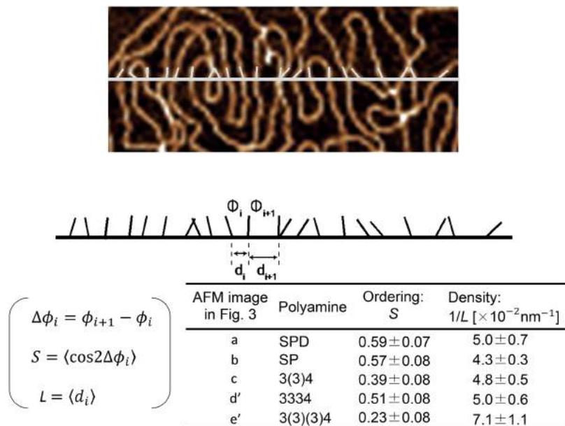
FIG. 6. Schematic representation of the procedure used to evaluate the order parameter  $S$  and the density  $1/L$  from AFM images.  $S$  and  $1/L$  are calculated from the equations  $S = \langle \cos 2\Delta\phi_i \rangle$  and  $L = d_i$ , where  $\langle * \rangle$  is the ensemble average. The lower table shows  $S$  and  $1/L$  based on the AFM images in Figs. 3(a)–3(c), 3(d'), and 3(e').
