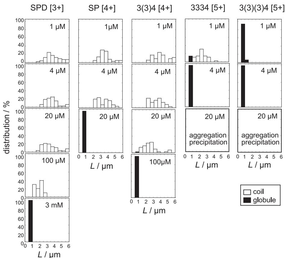
FIG. 2. Distribution of the long-axis length  $L$  of T4 DNA in solution at various polyamine concentrations. The DNA concentration is 0.1  $\mu\text{M}$  in nucleotide units.
