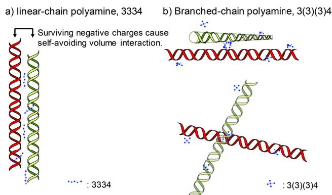
FIG. 7. Schematic illustration of different modes of interaction between double-stranded DNA and polyamines just before compaction. (a) Self-avoiding volume interaction between DNA segments induces parallel alignment; (b) high basicity of 3(3)(3)4 promotes “bridging” of DNA segments even when repulsive negative charge survives.
