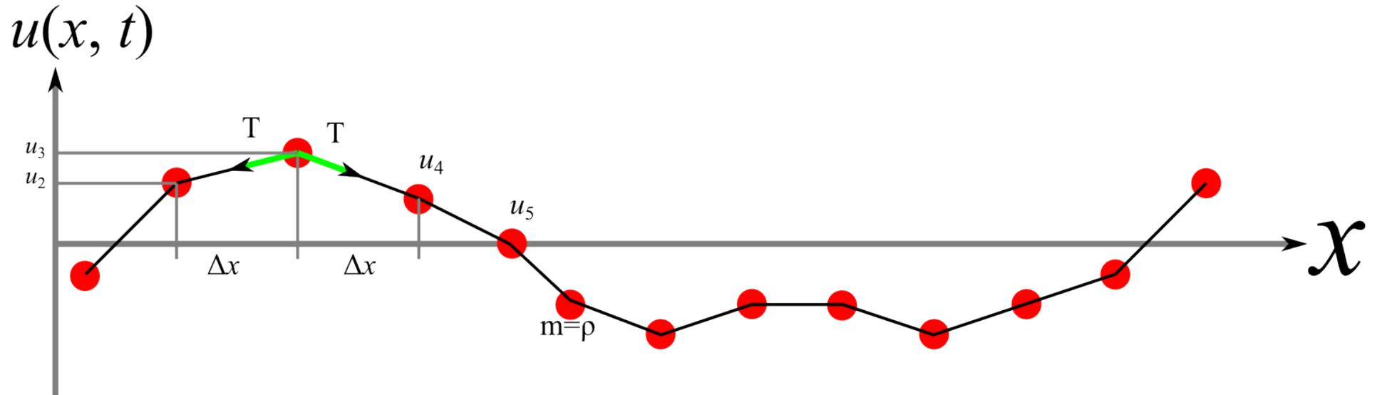
$$F_u = T \frac{u_{i-1} - u_i}{\sqrt{(\Delta x)^2 + (u_{i-1} - u_i)^2}} + T \frac{u_{i+1} - u_i}{\sqrt{(\Delta x)^2 + (u_{i+1} - u_i)^2}} \quad (i = 1, 2, 3, \dots, N)$$
